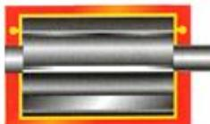
Unlike other compressors, the absence of axial thrust in the Mattei vane compressors eliminates the need for rotating bearings. This allows
