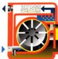
The three-stage system for separating the oil from the air assures the residue oil level in the compressed air remains lower than 3 ppm. This system offers low oil consumption and a
